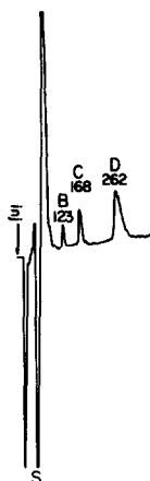
Fig. 10. Chromatogram of water extract from sample 1. The chromatographic conditions are given in Table I. Peaks: S = system peak; B = nitrate; C = chlorate; D = sulfate.
